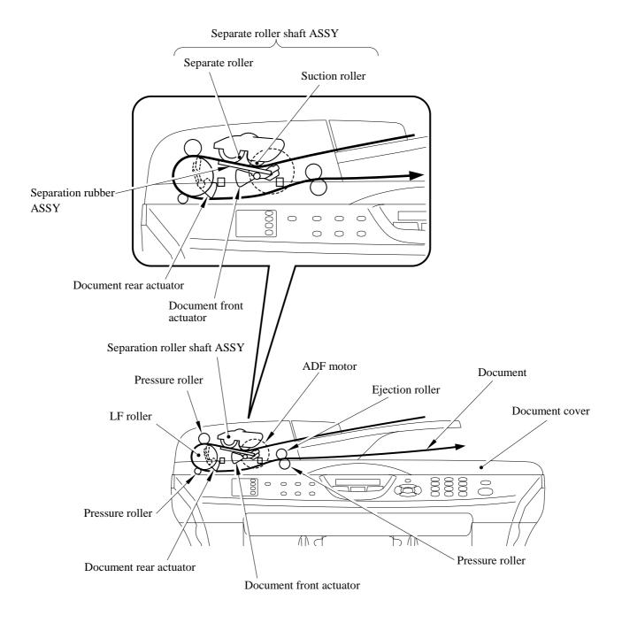
This scanner mechanism supports a dual scanning system: ADF scanning and flat-bed scanning. They automatically switch to the former at the start of a scan operation if the document front sensor inside the ADF detects a document.
