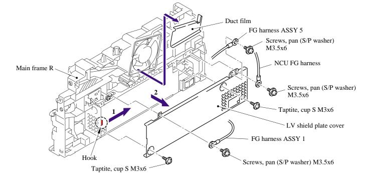
(7) Remove the LV insulation sheet.
