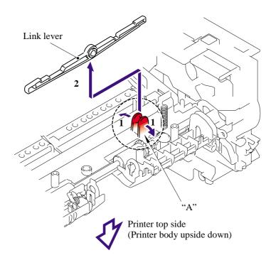
**NOTE**: When re-assembling the link lever, insert the end of the link lever into the main frame L referring to the figure below.
