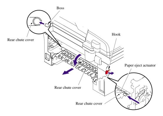
(2) Remove the paper eject actuator and the eject actuator spring.
