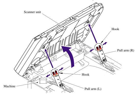
(3) Remove the pull arm springs and remove the pull arms (R,L) from the pull arm guides.
