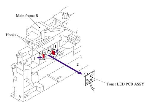
(2) Remove the LED holder from the toner LED PCB ASSY.
