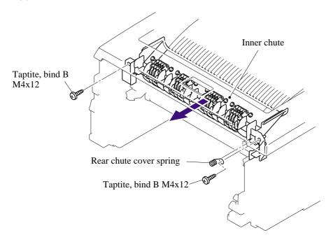
**NOTE**: Re-assemble the inner chute while pushing onto the pinch roller of the inner chute with the eject roller of the joint cover ASSY.
