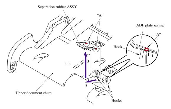
(17) Remove the separation rubber from the ADF plate spring.
