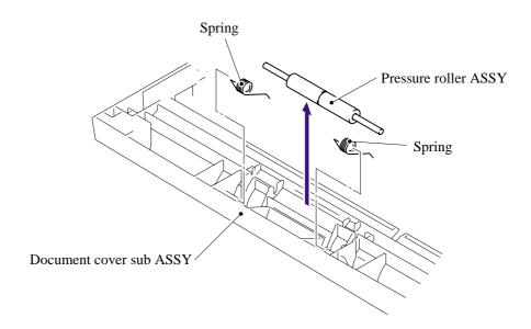
(43) Remove the two pressure rollers from the pressure roller shaft.
