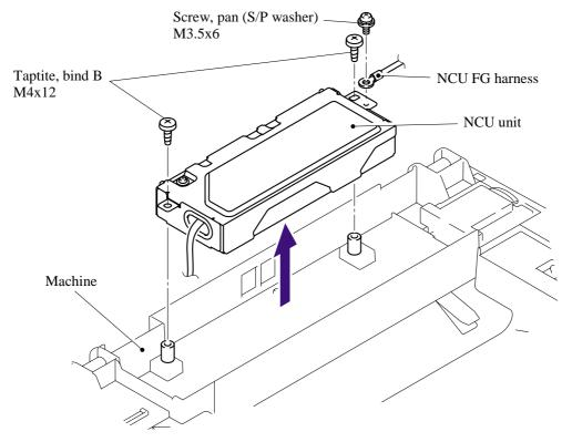
(2) Remove the one pan (S/P washer) M3.5x6 screw from the NCU shield cover to remove the NCU shield plate.
