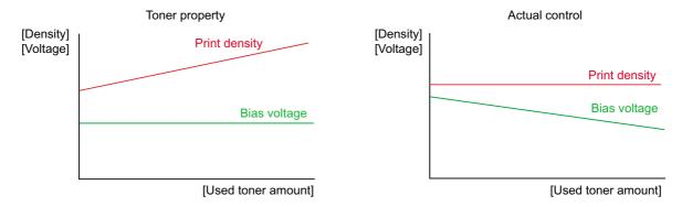
To always obtain a print result of a constant density, the printer counts the number of print pages immediately after the toner cartridge is replaced and changes the bias voltage according to the accumulated number of prints with the toner cartridge.
