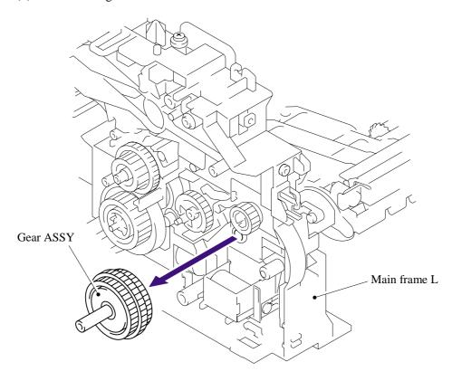
**NOTE**: The gear ASSY contains the small gears. Be careful not to lose them by disassembling the gear ASSY.
