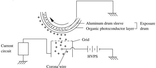
The primary charge uses a corona wire, but since the drum is positively charged, only less than 1/10 of the usual quantity of ozone is generated compared with the negatively charged drum. The level of ozone expelled from the printer is therefore not harmful to the human body. Applicable safety standards have been complied with.
