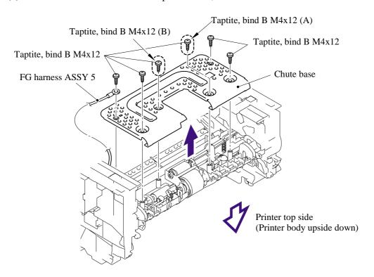
**NOTE**: When re-assembling the chute base, check that the bind B M4x12 taptite screws (A) and (B) shown in the figure above are secured correctly.
