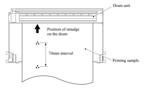
(2) Turn the drum gear by hand while looking at the surface of the exposure drum.
