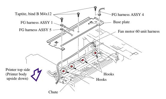
(3) Release the harness from the hook, and then remove the fan motor 60 unit from the main frame R.
