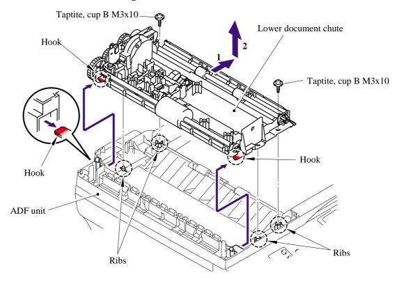
(20) Release the hook on the ADF unit and remove the ejection roller ASSY.
