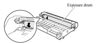
(3) Wipe the surface of the exposure drum with a cotton swab until the dust or paper powder on the surface comes off.
