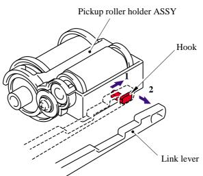
**NOTE**: The pickup roller holder spring is assembled on the bottom of the pickup roller holder ASSY. Be careful not to lose the spring.
