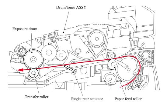
The regist rear actuator in the path from the feed roller to the transfer roller controls the first print position on the paper. The printer starts transferring an image when a definite time passes after the paper is passed through the regist rear actuator.
