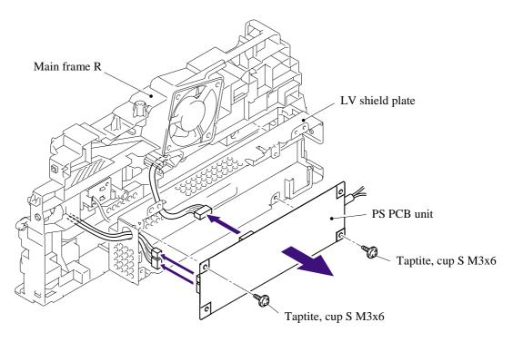
**NOTE**: When disconnecting the connectors, disconnect the regist sensor PCB connector and toner LED PCB unit ASSY connector first, lift up the PS PCB unit from the LV shield plate, and disconnect the main PCB connector.
