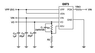
1. VO =  $\frac{0.8 \text{ (R1+R2)}}{\text{R2}}$  Volts, R2<120k $\Omega$  is recommended
