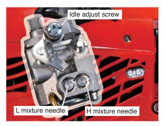
1. Start and warm engine for 1 minute alternating engine speed between WOT and idle every 5 seconds. Turn H mixture needle anticlockwise until engine speed drops to approx. 12,000 r/min at WOT.
