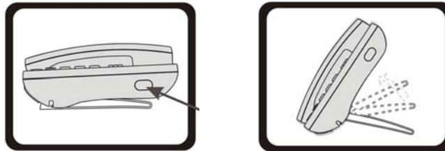
**Press and hold the button of right side to change the stand mount angle.**
